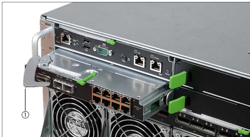
Figure 37: Installing a connection blade
